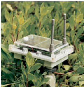
Sense and sensibility: One of Kevin Delin's sensor web pods measures soil and climate conditions in a garden. The gray antennas let it communicate with other pods in a wireless network to relay and process data. (Photograph by Dave Lauridsen)
