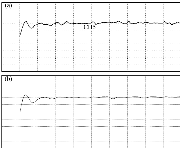
Figure 9 The responses of I_d . (a) The response of I_d in the real system; (b) the response of I_d in the simulation system.
